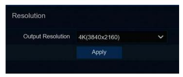
If you connect to a 4K HDMI monitor, you are able to choose max. 4K (3840x2160) resolution. If you connect a VGA monitor, do not choose the resolution larger than 1080P(1920x1080).
