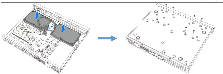
3. Put the upper cover back carefully, and fix the cover with screws.
