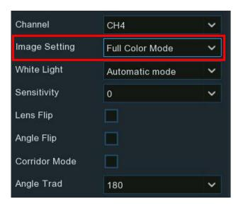
Full colour camera includes not only IR LEDs, but also white light LEDs. You're able to determine the operating mode of the lights:
