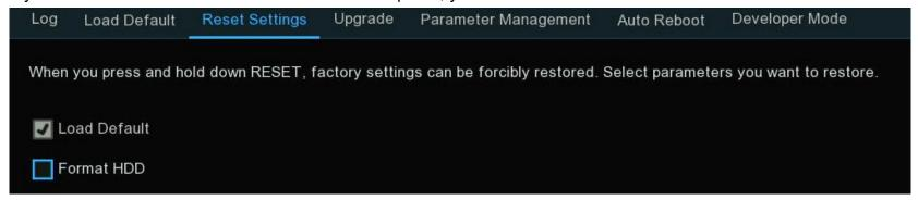
By default, when you press and hold 10 seconds on the reset button with a small pin till the NVR beeps, the NVR will restore default settings. You can tick the checkbox to format HDD if needed.
