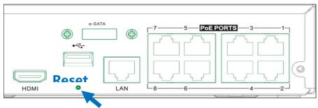
Press and hold 10 seconds on the button with a small pin till the NVR beeps.
