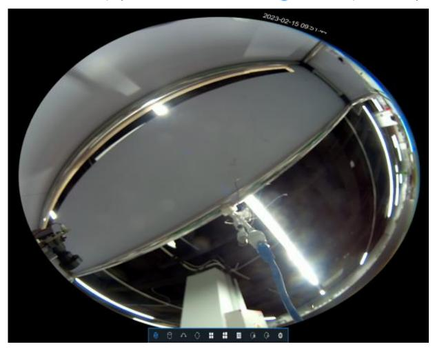
On the fisheye-mode operation page, click the button on the toolbar at the bottom to open the menu for setting the fisheye camera installation mode. Then, select the mode in accordance with the actual installation mode, and save the setting to make it take effect.
