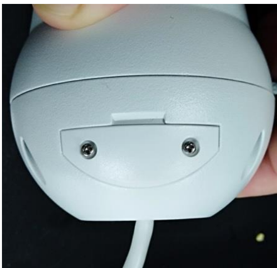
Image above shows how to access reset button on cameras with turret housing
