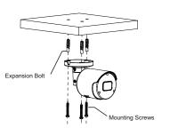
Insert three expansion bolts in place into the ceiling and fix the equipment with three mounting screws.
