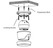
Fix the pedestal by drilling locking holes around the sticker and inserting three expansion bolts into the holes and fastening it with three locking
